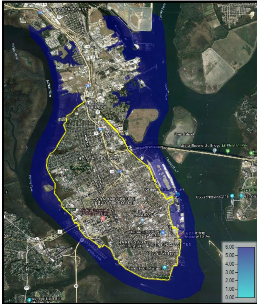
Figure 8.1.5.1. 12' NAVD88 wall versus a 6' NAVD88 exterior WSE with no rainfall
